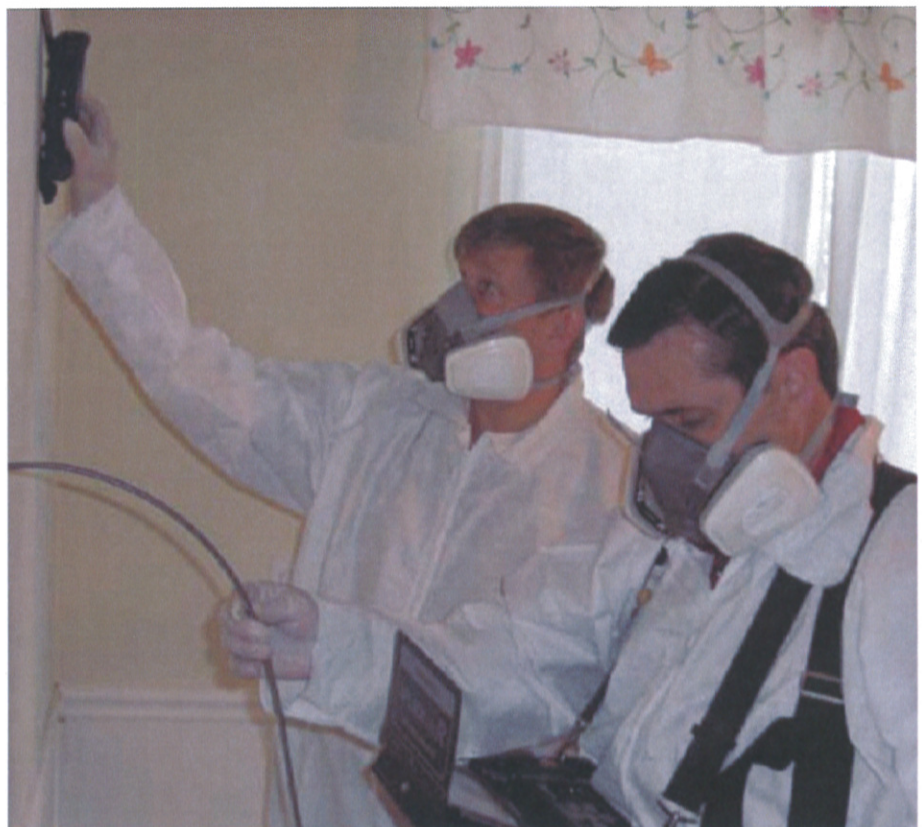
(right) Using high-tech forensic equipment, inspectors can determine if there are problems with the drywall without having to knock down a wall.
